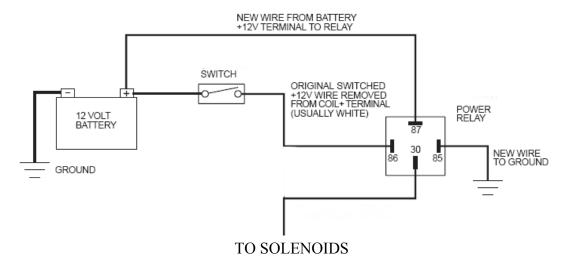
SOLENOID WIRING: The wire from the battery to the arming switch can also have a push button style thumb switch for the activation or you can use the switch as the arming switch and then use a micro switch for wide open throttle activation.
