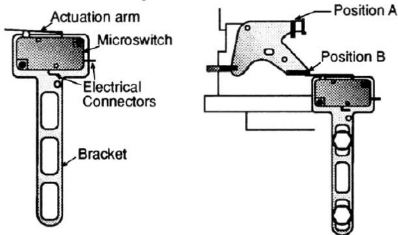
1. Connect the bottom terminal of the micro switch to the middle of the arming switch.
