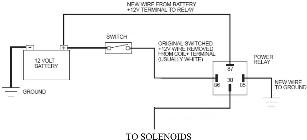
**SOLENOID WIRING:** The wire from the battery to the arming switch can also have a push button style thumb switch for the activation or you can use the switch as the arming switch and then use a micro switch for wide open throttle activation.
