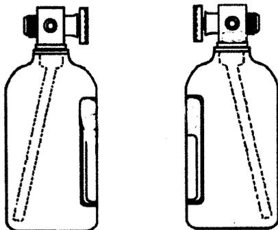
**Figure 3 Nitrous Bottle Mounting Orientations**
